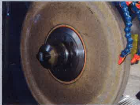
Automatic balancing system for grinding wheel, incl. display
